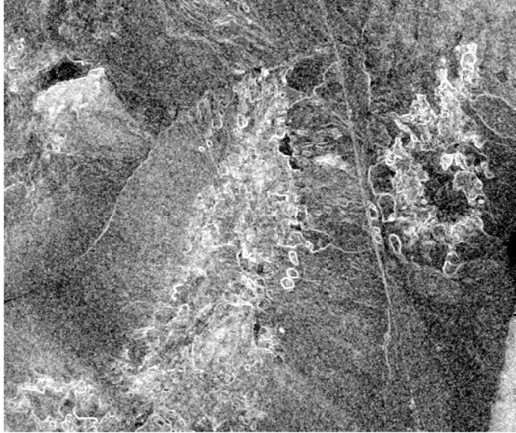
Figure 10. Sample results from the Auto-Correlogram process for the 1997 AVIRIS scene of Cuprite, using the 1.98 to 2.467 \mu\text{m} band subset. Pixel gray levels represent the average spectral angle between each pixel and its adjacent neighbors (with contrast stretch applied). Spectrally uniform areas appear dark, while bright pixels separate areas with contrasting spectral characteristics.
