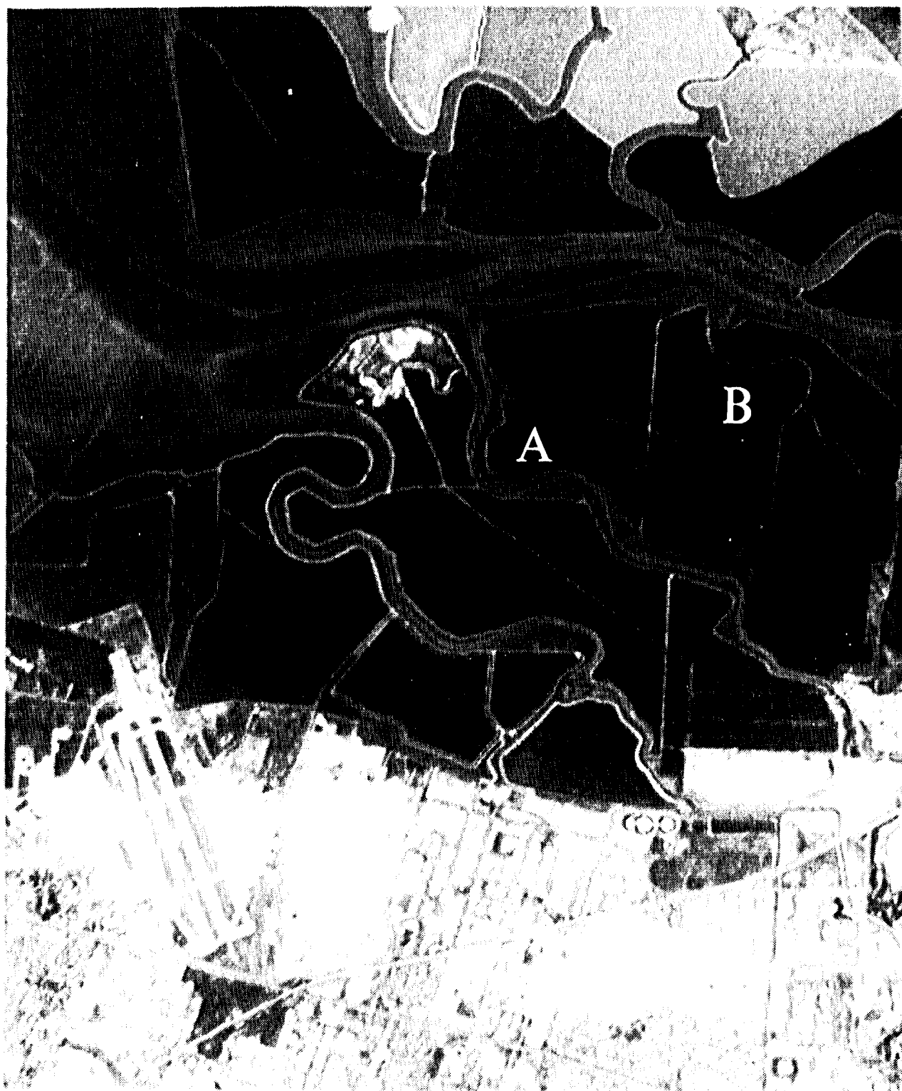
Figure 1. AVIRIS image (single band) of salt ponds near NASA Ames Research Center. Radiance data are from 675.7-684.9 nm (band 30) which covers the red absorbance feature of chlorophyll a .
