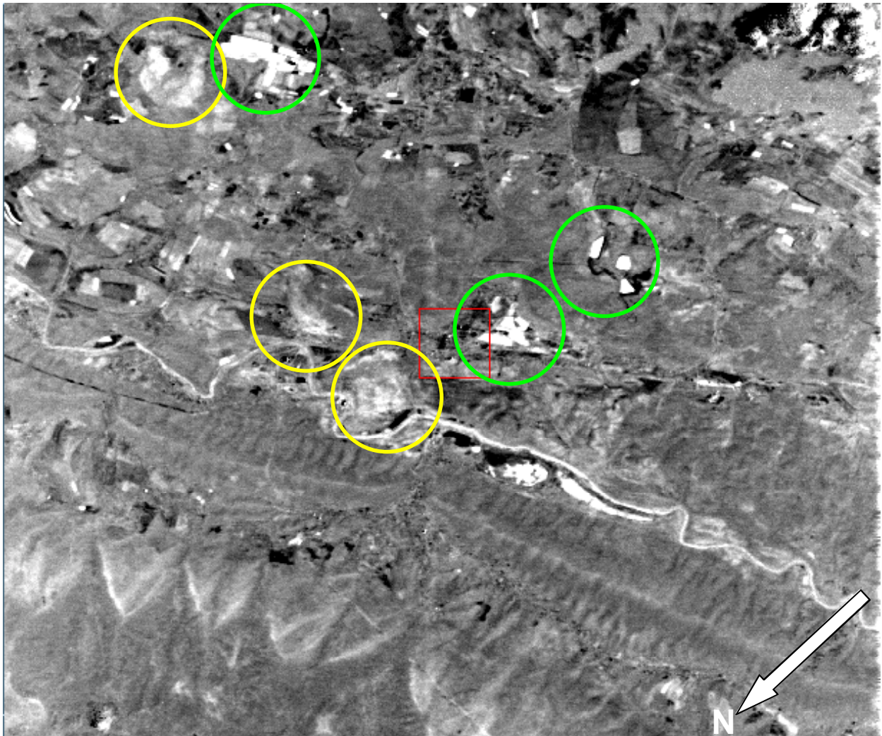
Figure 9: MNF (minimum noise fraction) transform of the Saltville reflectance image. The transform picks out spectrally unique regions. Note that the same regions of interest are highlighted by both techniques (yellow circles), while the MNF emphasizes additional regions (green circles).
