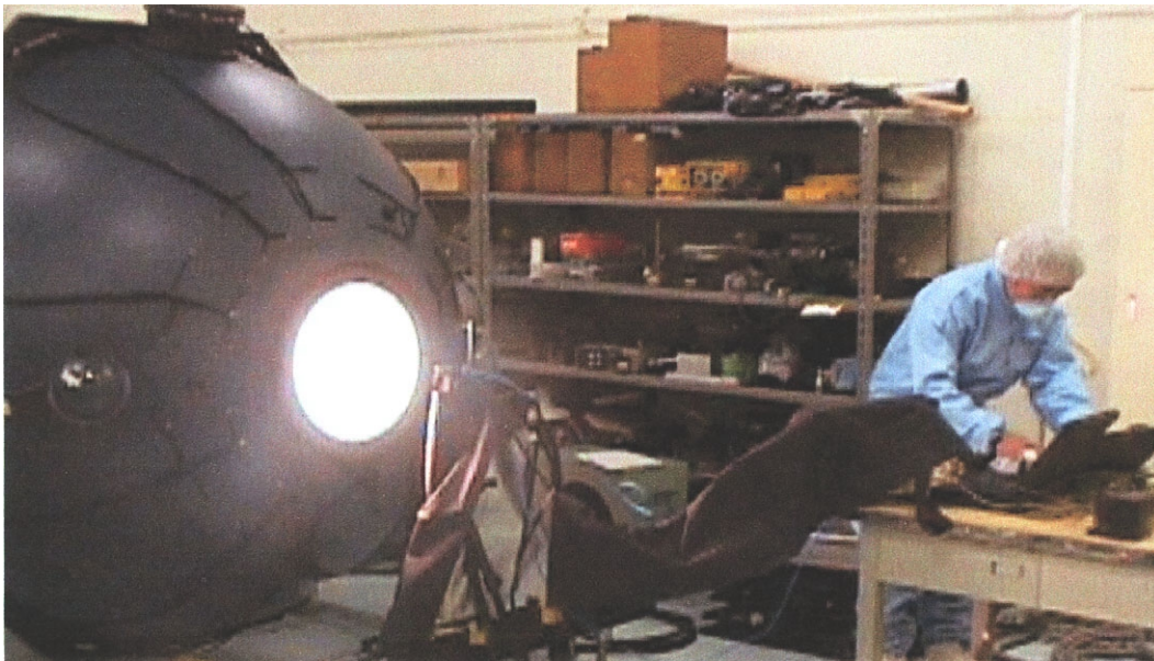
Figure 5. Test configuration of absolute calibration accuracy of the portable calibration source (right)
