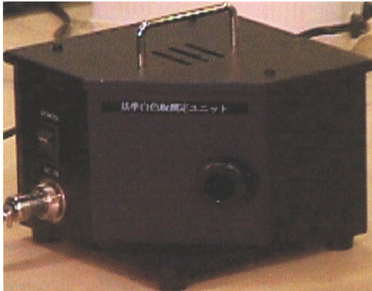
Figure 3. Outlook of the proposed portable calibration source
