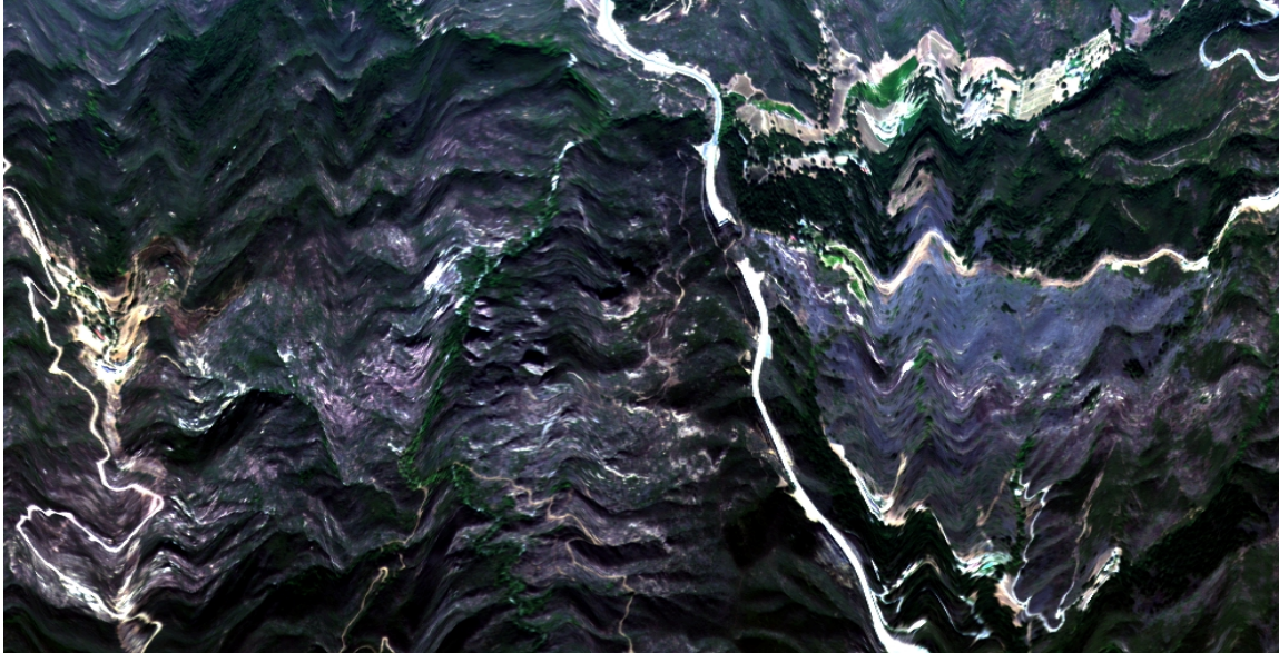
Figure 9. Ungeorectified AVIRIS low-altitude data acquired over the Santa Monica Mountains, California, on the 5 th of October 1998.
