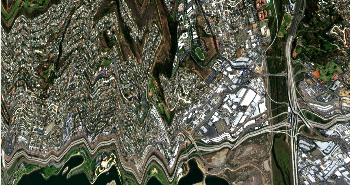
Figure 11. Ungeorectified AVIRIS low-altitude data acquired over portions of San Diego, California, on the 12 th of October 1999.
