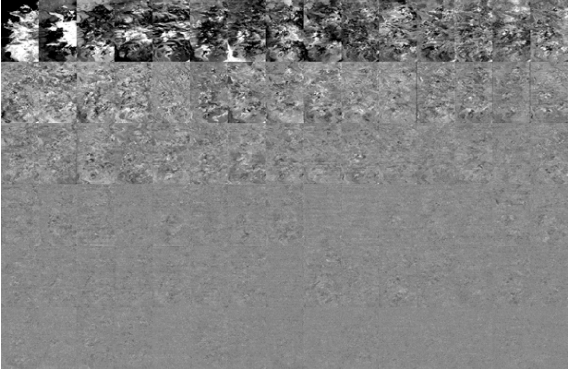
Figure 3. A grid of 16 \times 6 output MNF transform images from the baseline AVIRIS Cuprite, Nevada, 1998 data set. Spatially coherent features are an indication of information. Spatially coherent features are largely gone above MNF image 48.
