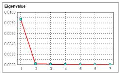
Figure 10. The K-L transformation eigenvalues indicate that most of the information provided by the seven indices is captured in the first principal component that, being a linear combination of all seven indices, captures most of the scene variance.
