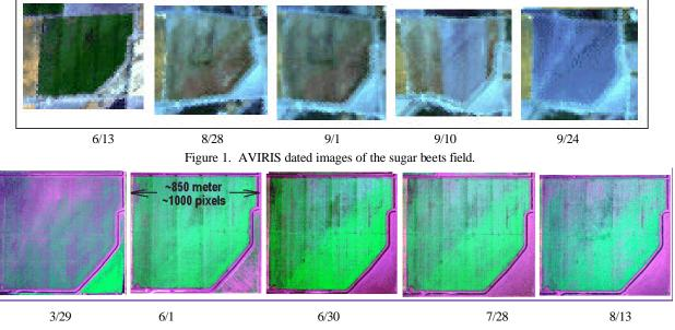
Figure 2. SAMRSS dated images of the sugar beets field. The 1st image shows primarily bare soil. The 2nd and 3rd show increased level of vegetation, while the 4th and 5th show an increase in senescing vegetation from the northwest corner moving later towards the southeast corner. (In this false color image using, B=548 nm, G=658 nm, and R=850 nm, vegetation appears green and soil is purple)
